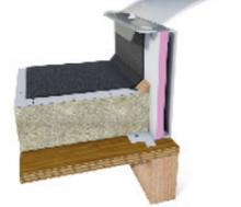
Flat board insulation (Aluminium kerb)
