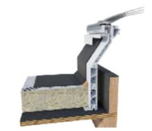
"Sleeving over" existing rooflight kerb
