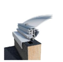
Fixing direct to an existing or new builders kerb.
